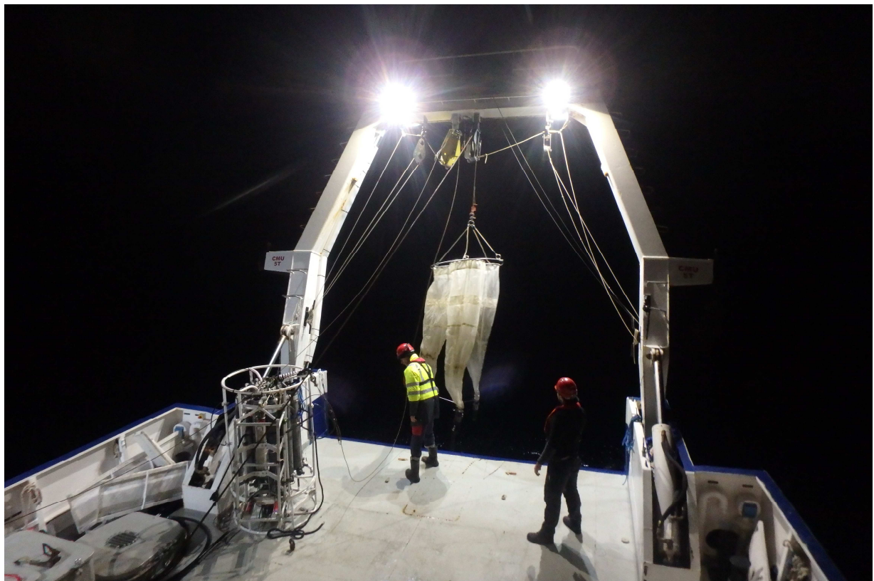
Deployment of the triple WP2 zooplankton net from the deck of the R/V Téthys II for the MOOSE DYFAMED program.
